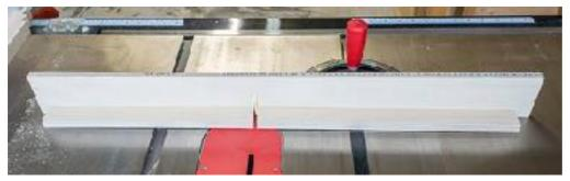
This jig serves two purposes: one is to limit or prevent blowout on the back face of the cut. The other is that this will provide a very exact location to line up your cuts. Note that I've placed a line on the banding where I want the cut and an "x" on what side of the line I want to do the cut.
