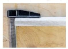
But there are other clamps that have arches or a raised head on their fixed jaw, meaning that if a clamp is resting on that pad, the clamp will rock inward.
