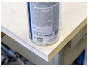
To round the corners, I grabbed an appropriately sized spray can in my shop, traced around the edge and cut it with my jig saw. This was cleaned up with my disk sander. After some sanding I used a ¼" roundover bit to round over the hand hold and the top region of the centre section. Make sure to stop the rounding over on the edge before the shelving starts. Sand by hand until smooth.
