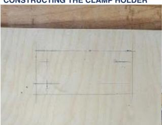
After cutting the parts to size, mark out the location of the four 1" Forstner bit holes.
