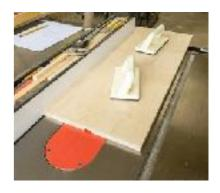
If you are not dead-on-centre in this cut (which is actually very hard to do), be sure to maintain the alignment to each other. To check, hold the boards against each other so the grooves face each other. If the grooves don't line up, flip one board 180 degrees. If this corrects the problem, mark the boards accordingly so it's easier when you do the final assembly later.
