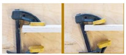
The facing placed on each shelf (1/8" proud of the top surface) is high enough to help support most clamps very well. Otherwise, the clamps with a high arch from the fixed jaw require a second lower shelf to "catch" the clamp's bar from swinging in any further. In the image above, the first and third clamp depends upon the lower shelf while the second and fourth are resting on the shelf's hard wood facing.
